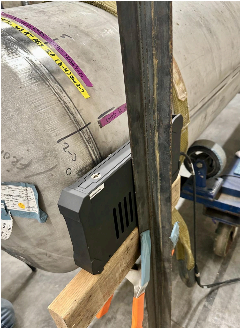
Figure 2: Image shows Pacific NDT's Flat Panel Digital Radiography Solution mounted on a curved pipe. Product Link: https://pacificndt.com/solutions/ndt-x-ray-machine-pix-pikena/
