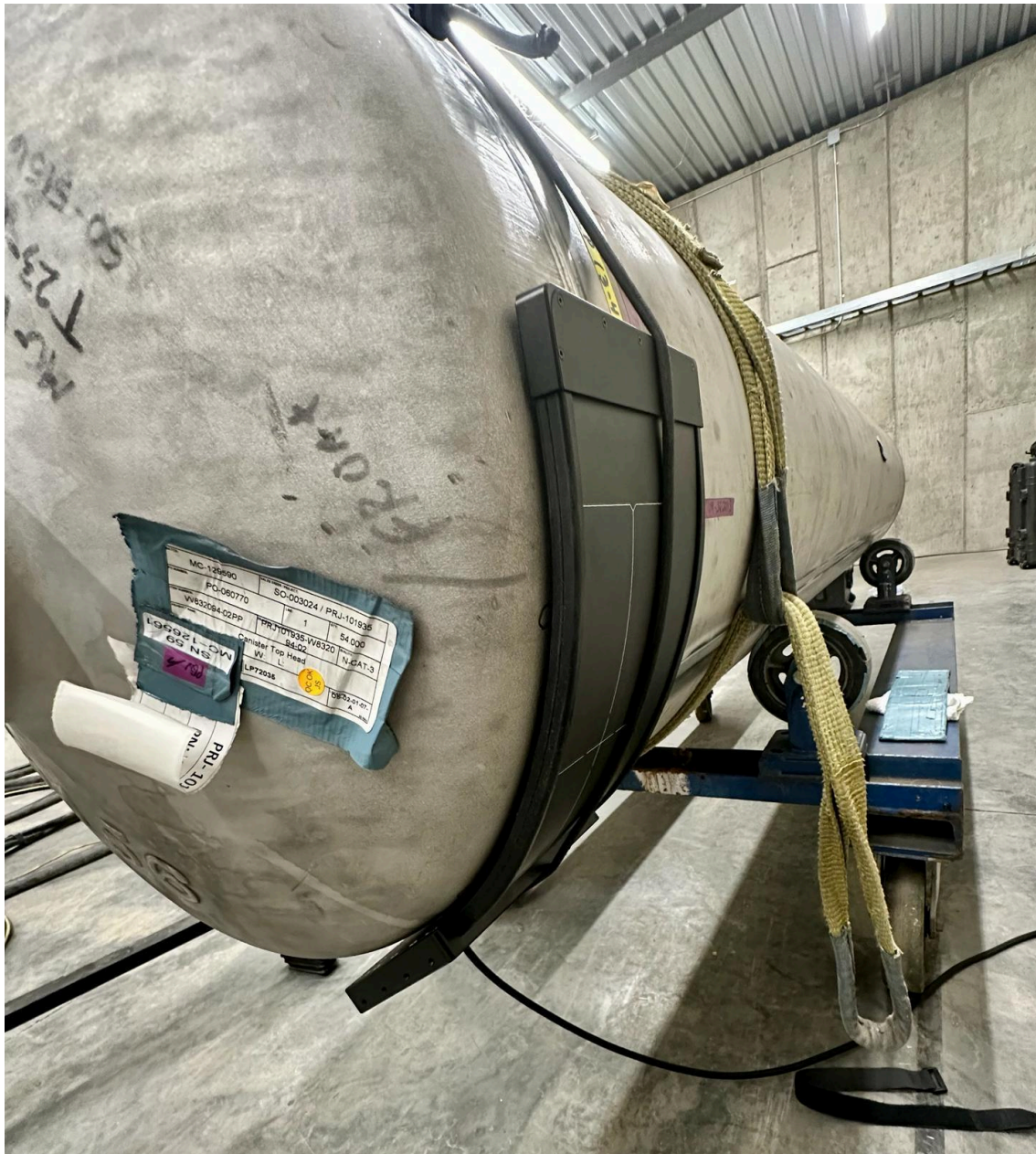
Figure 3: Image shows Pacific NDT's bendable/Flexible Digital Radiography Solution mounted on a curved pipe. Product Link: https://pacificndt.com/solutions/pix-417c/
