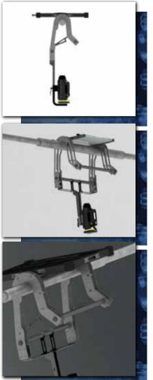
PiX Raven includes a state-of-the art digital detector inside our IP68 rated protective armor (Rhino), portable X-Ray, Air Pi Trigger Box all mounted on newly upgraded mount for inspecting sleeves and connectors. Our carbon fiber frame mounts on the powerline and is one of the safest methods to safely inspect conductor sleeves on power lines.
