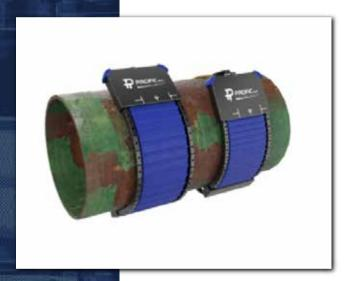
The PiX 417C is one of three rugged, bendable panel detectors (BPD) offered by PacificNDT. As indicated by its name, the PiX 417 features a 4" wide by 17" long active sensor area, making it ideal for imaging cylindrical vessels and pipelines. Built for field use in extreme NDT environments, the PiX 417C delivers outstanding performance with Pulse Potential X-Ray, Constant Potential X-Ray, and Gamma Ray sources.
